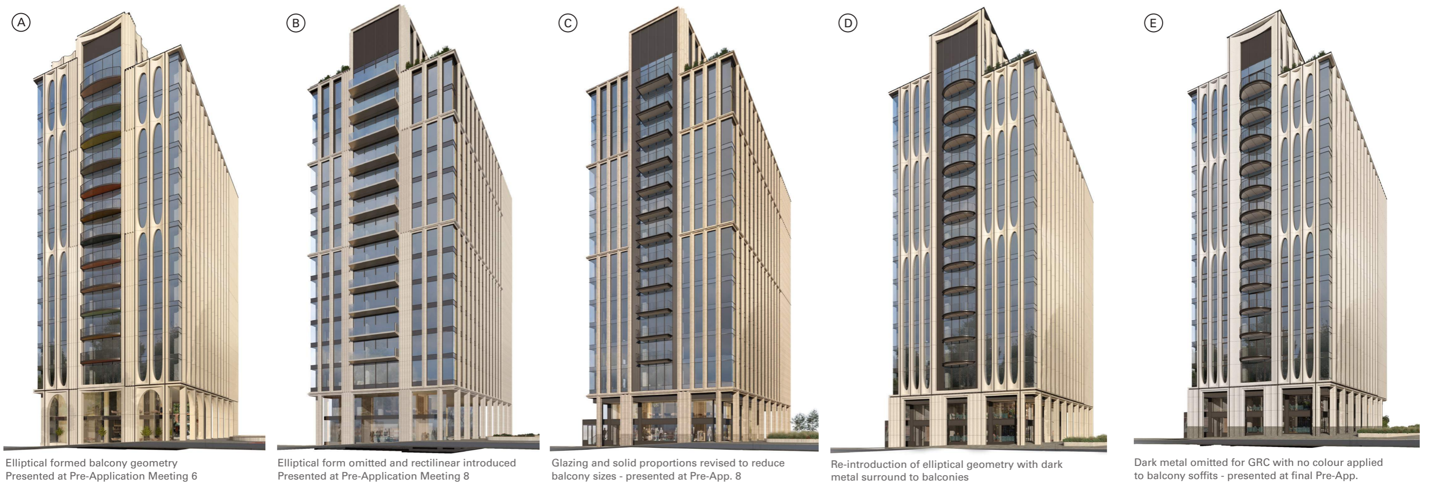
Fig. 3.70: Illustrative visualisations of the evolution to the east elevation and balcony provision to Newcombe House
