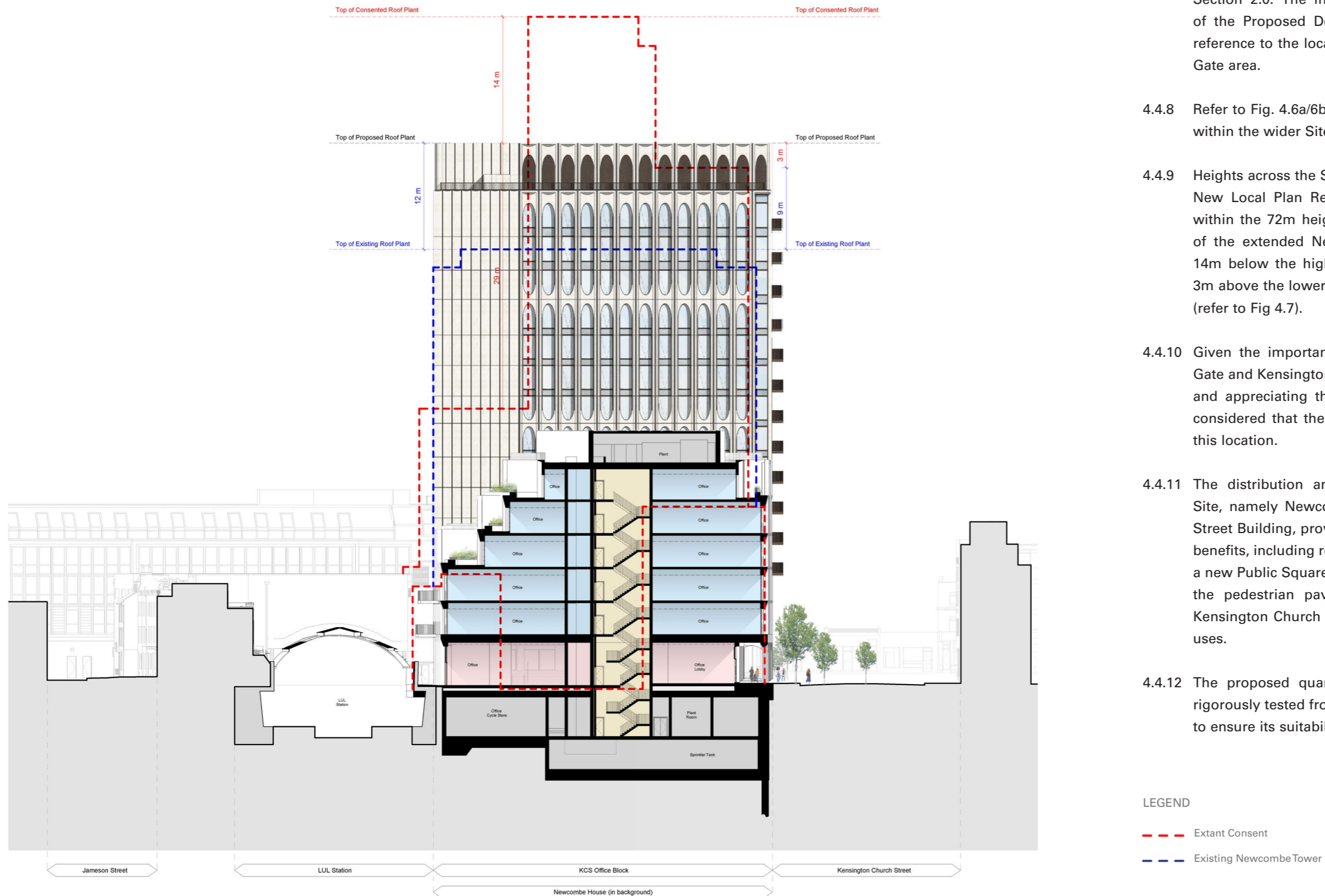
Fig. 4.7: Illustrative diagrammatic east-west section of proposal with consented scheme red outline and comparative dimensions
