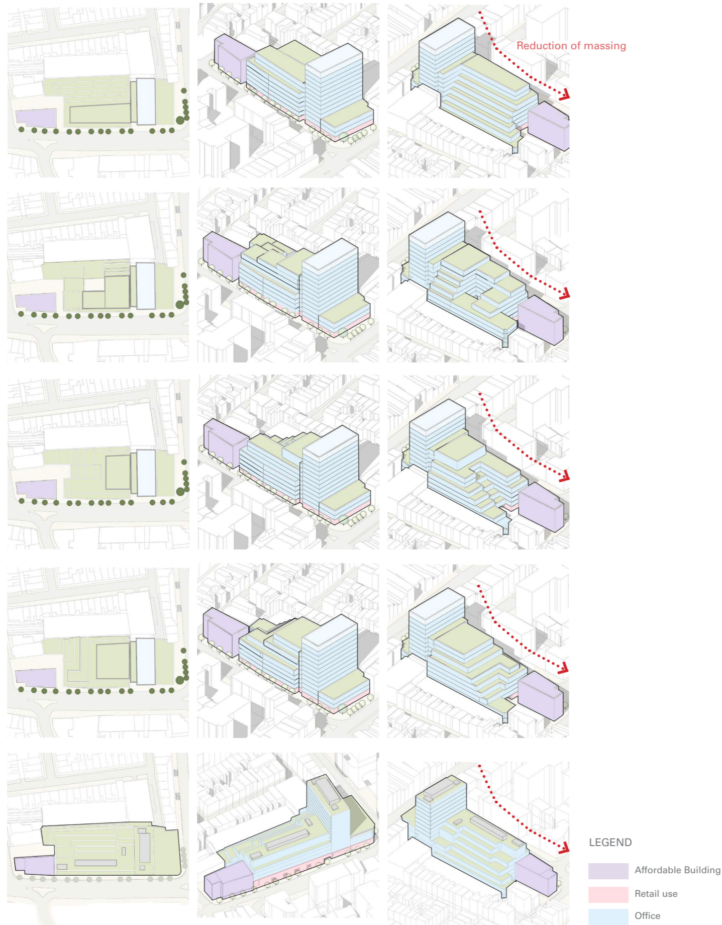
Fig 3.7: Early diagrams exploring how the mass of the Site could be distributed
